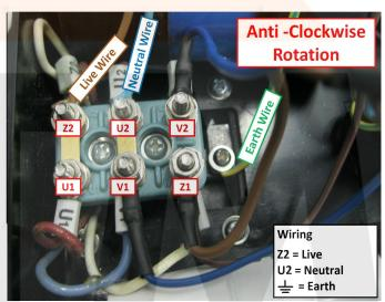
Diagram is also located under the terminal box cap. We recommend contacting an electrician if you are unsure about the wiring.
