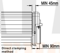
Ensure that there is at least 45 mm from the edge of the curtain to the edge of the bracket. If the roller door drum is on the edge of the curtain or is a smaller diameter, additional clearance may be required.
