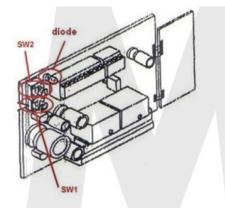
1. Open your motor, and try and find the receiver. If your receiver is in a case, then remove the casing.
