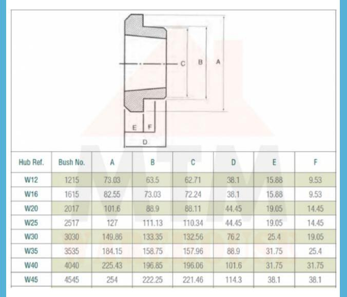
**Includes**: 1 x *W12* Weld on Hub + *1215* Taper Lock Bush to suit (Select from drop-down box)
