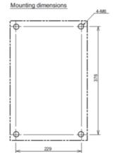
Higher Resolutions Technical Drawings and Specifications can be seen in the listing Images and in the manual.
