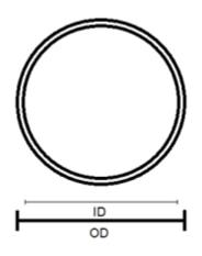
**How To Measure** ID(mm) x Thickness(mm) eg. ID(11mm) x Thickness(1mm) OD(mm) = ID(mm) + 2 x Thickness(mm)
