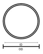
**How To Measure** ID(mm) x Thickness(mm) eg. ID(5mm) x Thickness(3mm)
