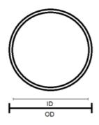
How To Measure ID(mm) x Thickness(mm)
