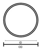
How To Measure ID(mm) x Thickness(mm)
