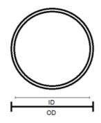
How To Measure ID(mm) x Thickness(mm)
