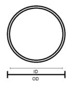
How To Measure ID(mm) x Thickness(mm)
