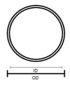
How To Measure ID(mm) x Thickness(mm)
