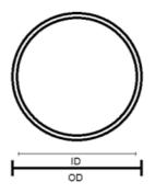
How To Measure ID(mm) x Thickness(mm)
