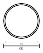
How To Measure ID(mm) x Thickness(mm)
