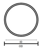
How To Measure ID(mm) x Thickness(mm)
