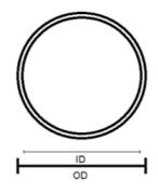
eg. ID(5mm) x Thickness(3mm) OD(mm) = ID(mm) + [2 x Thickness(mm)] 11mm = 5mm + (2 x 3mm)
