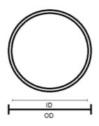
How To Measure ID(mm) x Thickness(mm)
