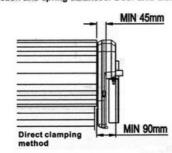
Ensure that there is at least 45 mm from the edge of the curtain to the edge of the bracket. If the roller door drum is on the edge of the curtain or is a smaller diameter, additional clearance may be required.
